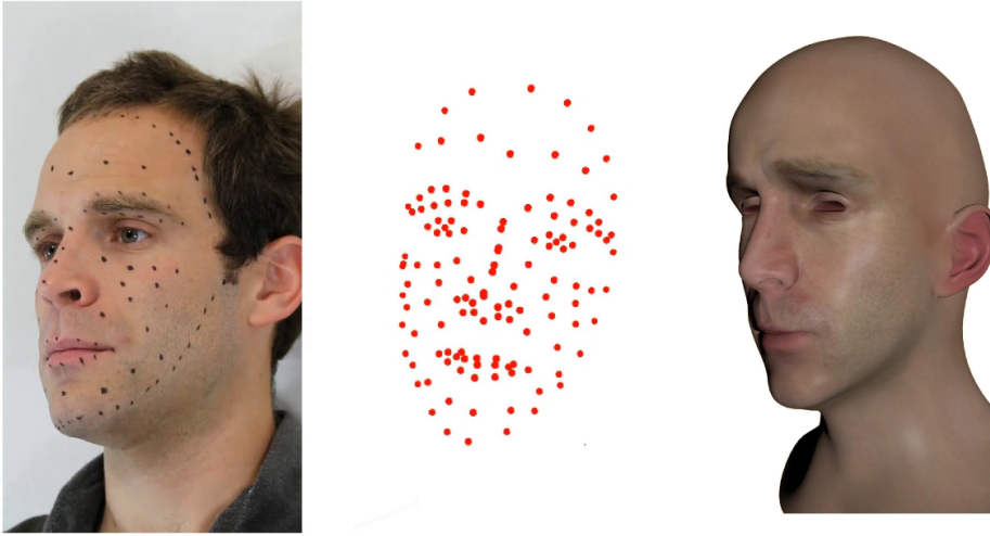
Figure 4.1 – Our performance capture setup. We use marker points tracked from an actor’s performance to animate a physical system built from user-specific blendshapes.
